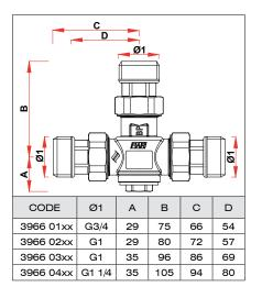
Body: brass CW617N - CB753S O-ring: EPDM Spring: Stainless steel AISI302 Shutter: PSU plastic material
