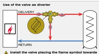
Install the valve placing the flame symbol towards the heat generator.
